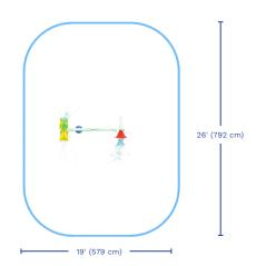
**Flow** 10-13 GPM 38-49 LPM Pressure 5-6 PSI 0.3-0.4 BAR
