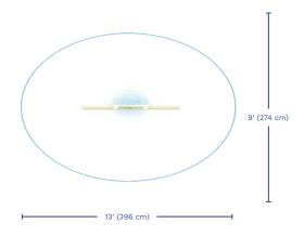
**Flow** 5-10 GPM 18.9-37.8 LPM Pressure 10-25 PSI 0.7-1.7 BAR
