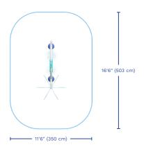
**Flow** 10-14 GPM 37.8-52.9 LPM Pressure 10-12 PSI 0.7-0.8 BAR
